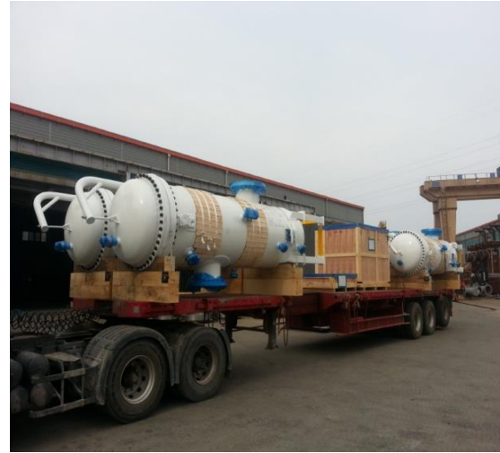
Fuel Gas Dust Filter Coalescer
